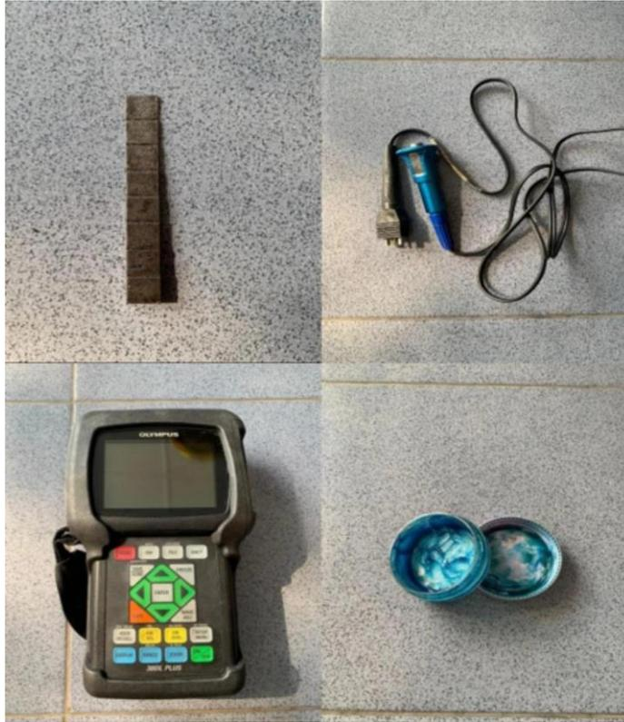
Gambar 2. Ultrasonic Thickness Gauge, Blok Kalibrasi, Couplant, dan Probe
