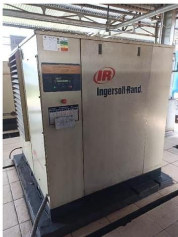
Gambar 1 *Screw Compressor* MM45
