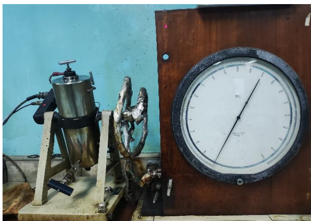
Gambar 3. Viskometer Rolling Ball
