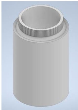
Gambar 4. Design Blast Joint 3D
