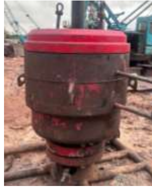
Gambar 3. Annular preventer 13 5/8 inci di Workshop PT Asrindo Citraseni Satria,
